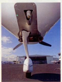
Though the canopy is slightly taller and beamier than those of previous DA40s, you'd have to look pretty closely to notice the comparative difference. Spotters can tell an XLS by the Power Flow exhaust system's large chrome external stack (below).
