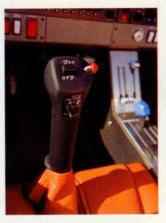
The DA40 control stick sits in your lap (above) and has a trigger-style microphone switch, plus electric pitch trim and autopilot disconnect switches. The G1000 (left) comes with an engine page on the MFD, plus a traffic information (TIS) and terrain awareness and warning system (TAWS)—all standard.
